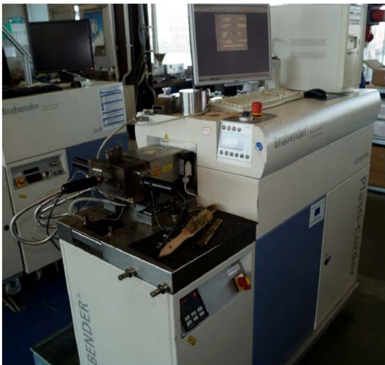
Screening der Compounds mittels Innenknetzer
